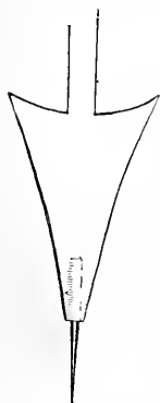
Fig. 381.—Manner of fastening Needle in Arrow-head.
